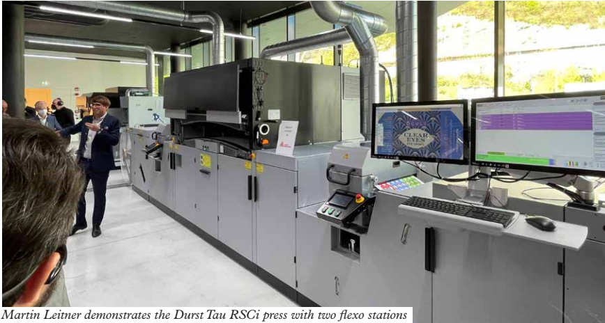
Martin Leitner demonstrates the Durst Tau RSCi press with two flexo stations
