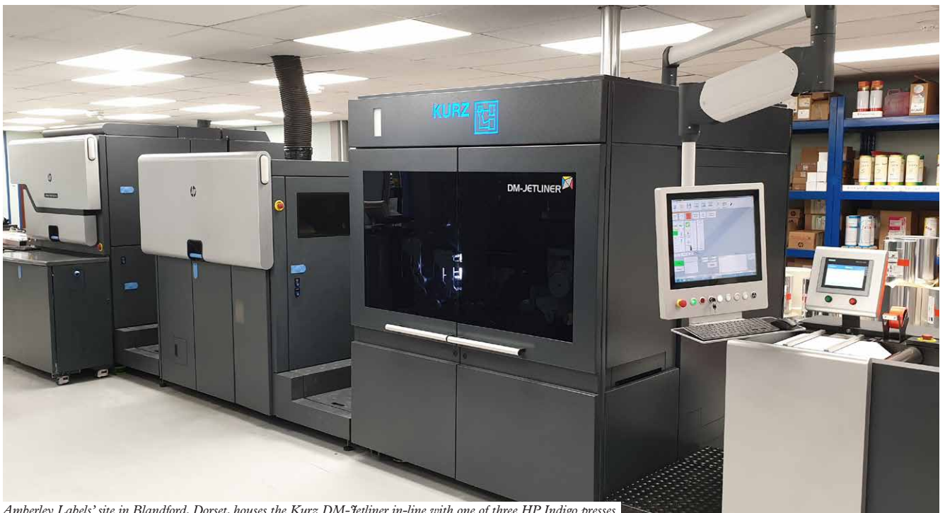
Amberley Labels' site in Blandford, Dorset, houses the Kurz DM-Jetliner in-line with one of three HP Indigo presses
