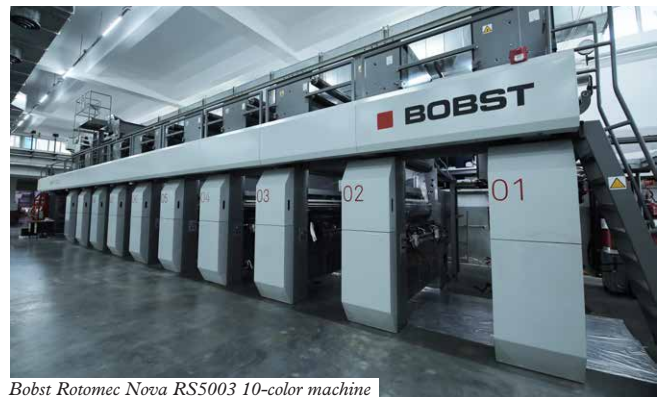
Bobst Rotomec Nova RS5003 10-color machine
