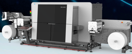
D1 New 4-colour direct digital roll to roll inkjet printing system
